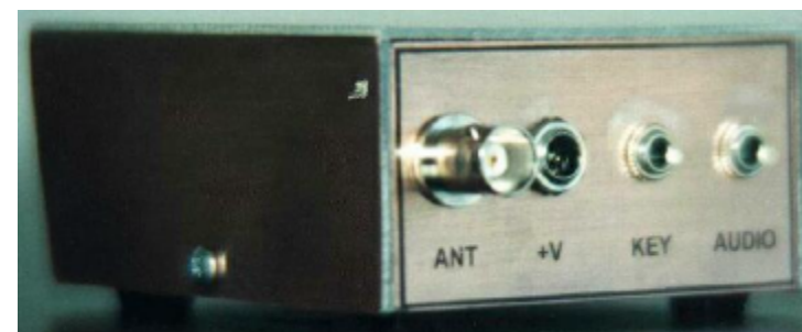
Figure 10: – Completed rear panel showing acetate labels applied.
